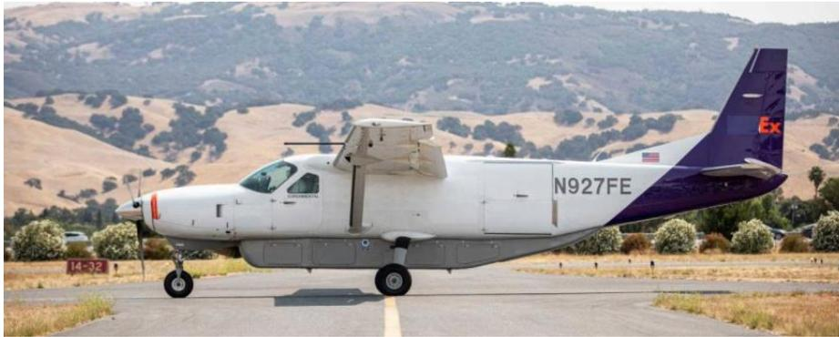
*Figure 2* Reliable Robotics Cessna Caravan converted LUCA (Thurber, 2020)
